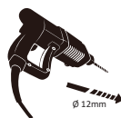
Electric drill + 12mm concrete drill bit
