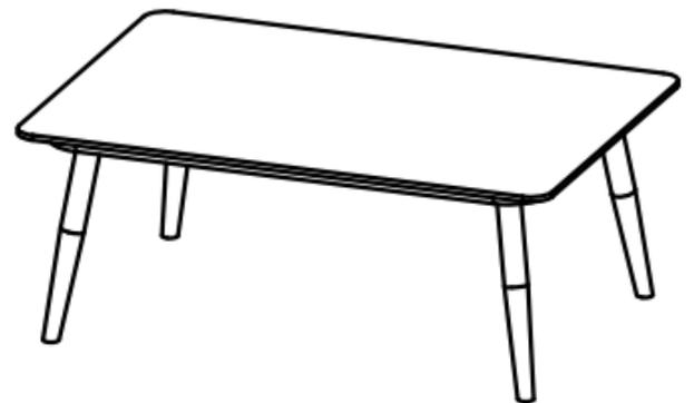
**STEP 1:** Attach leg frame (B) to table top (A) with bolts (C) & big flat washers (D), using Allen key (E).
