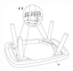
**STEP1:** Attach Leg1 (B) to the Frame (M), using the Bolt M6X20 (G) and Washer (H). Tighten the bolts and cover with the Plastic bolt cap (I)
