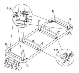
**STEP1:** Attach leg1 (B) ,leg2 (C), Center leg (D) to the Frame (A), using the Bolt M6X20 (G) and Washer (H).Tighten the bolts and cover with the Plastic bolt cap (I)
