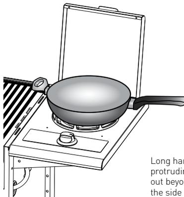
Long handles protruding out beyond the side burner can be dangerous.
