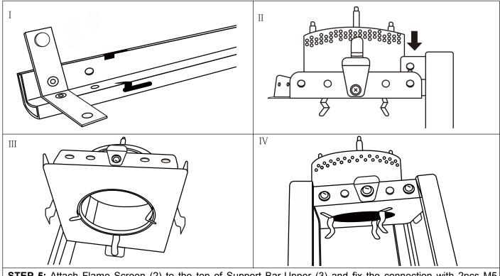
**STEP 5:** Attach Flame Screen (2) to the top of Support Bar-Upper (3) and fix the connection with 2pcs M5 screws and washers (BB), (See Figure I, II). Repeat this step and connect Flame Screen (2) to other 3 sets Support Bars-Upper (3). (See Figure III, IV)
