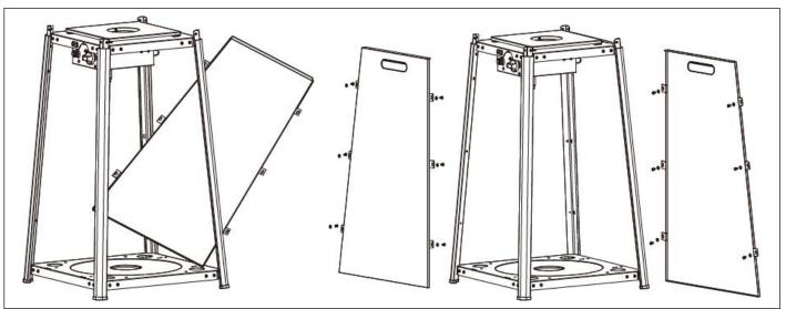
**STEP 3:** Obliquely insert and attach 2pcs Side Panels (12) and 1pc Rear Panel (10) into tank housing using 18pcs M5 self-tapping screws and washers (CC). Best affix two opposite sides first, fastening the screws diagonally.
