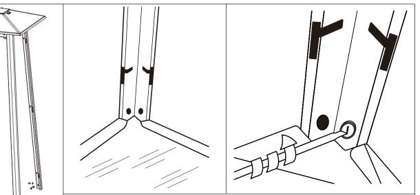
**STEP 7:** Place the whole upper parts to top of tank housing assembly. Make sure match the top ends of tank housing assembly with the bottom slot of Support Bar – Upper (3). Match the threaded holes and fix each connection with 2pcs M5 Screws and Washers (BB)
