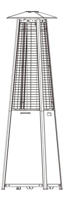
Model H1501 is 1.9m flame heater with stainless steel base Model H1502 is 1.9m flame heater with powder coated steel base Model H1505 is 1.9m flame heater with wicker base Model H1507 is 1.9m flame heater with LED panels and lights
