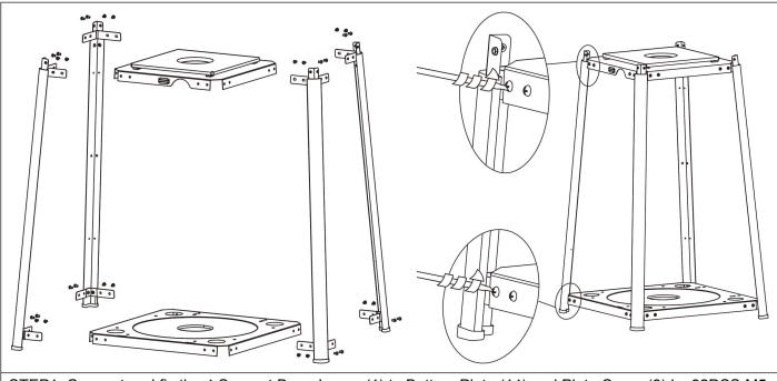
STEP1: Connect and fix the 4 Support Bar – Lower (1) to Bottom Plate (14) and Plate Cover (8) by 32PCS M5 screws and washers(BB)
