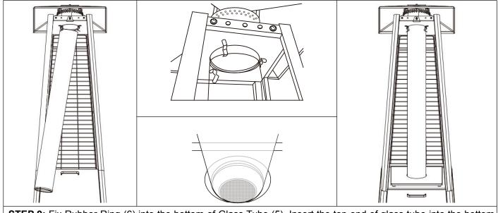
**STEP 9:** Fix Rubber Ring (6) into the bottom of Glass Tube (5). Insert the top end of glass tube into the bottom hole of Flame Screen (2) as much as possible. Keep glass tube vertically and sit it in the hole of Plate Cover (8). **NOTE: GLASS TUBE IS FRAGILE PART, PLEASE HANDLE GLASS TUBE CAREFULLY AND SLOWLY!**
