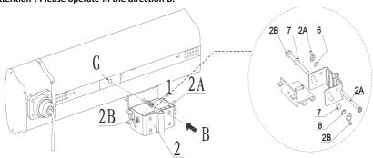
2.3.4: Drill two holes ( $\Phi$ 8\*40) on the wall, its distance is **55mm.** Install the hanger (No.4 in accessories list) on the wall with 2pcs M6\*60 (No.3 in accessories list) by the spanner.
