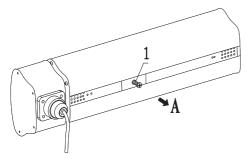
2.3.3: Fix the bracket set (no.2 of accessories list) on the heater By the screw M6x16, which is took off from the step 1.
