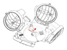
**3.** Open unit and attach around the parasol pole. Re-insert vertical thumbscrew and tighten fully home (do not overtighten).
