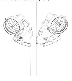
**4.** Slide unit up the parasol pole to the desired height (no less than 1.8m) and tighten large horizontal clamping thumbscrew.
