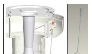
If for some reasons your ignition fails to deliver a spark, the heater can be started by inserting a lit match using supplied match holder through the burner hole (see left photo) while pushing the control knob in the "PILOT" position, which shall be performed by a qualified person
